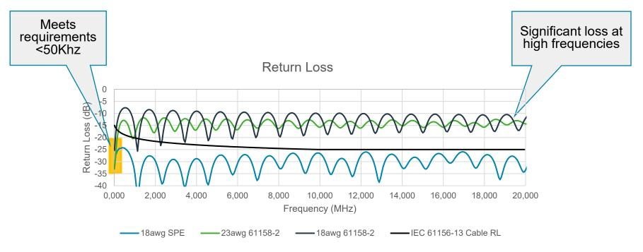
Legacy fieldbus cables have degraded performance at high frequencies
